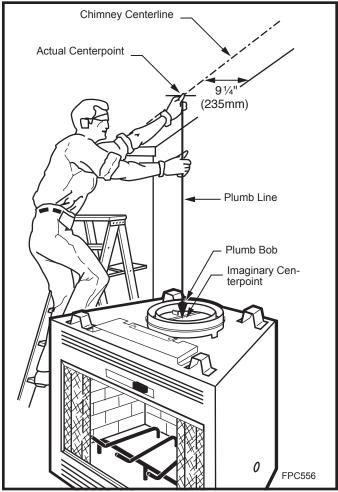
Fig. 11 Locate centerline of chimney with plumb line.
